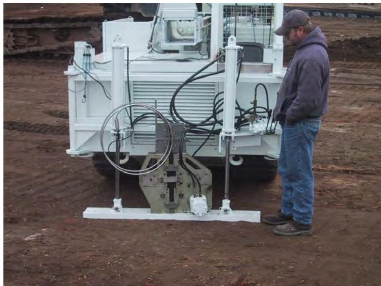
**Figure 14.** Mini CPT system with coiled rod delivery attached to small track mounted auger rig
