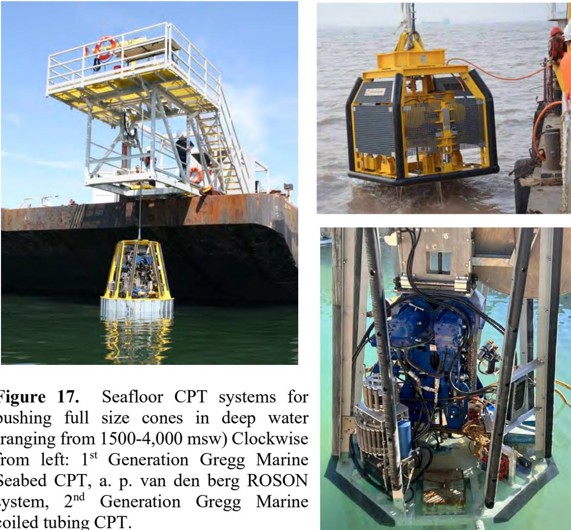
**Figure 17.** Seafloor CPT systems for pushing full size cones in deep water (ranging from 1500-4,000 msw) Clockwise from left: 1<sup>st</sup> Generation Gregg Marine Seabed CPT, a. p. van den berg ROSON system, 2<sup>nd</sup> Generation Gregg Marine coiled tubing CPT.
