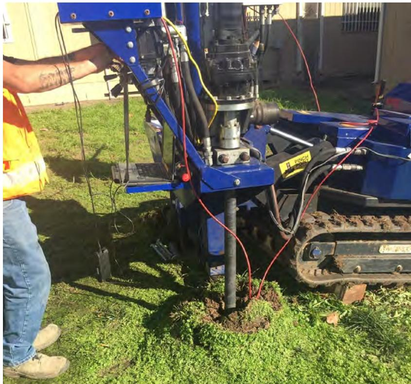
**Figure 12.** Small, anchored drill-rig unit
