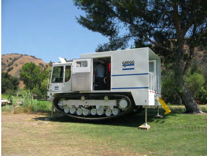
**Figure 11.** Track mounted 200kN (20 ton) CPT unit
