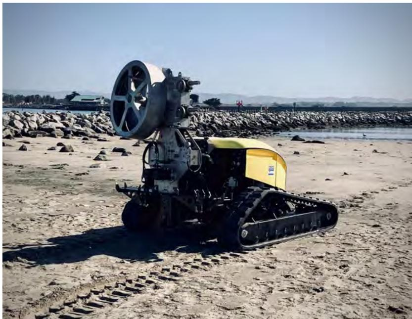
**Figure 18.** Gregg's Bumblebee remotely controlled, un-manned CPT system with 5cm<sup>2</sup> cone and coiled tubing
