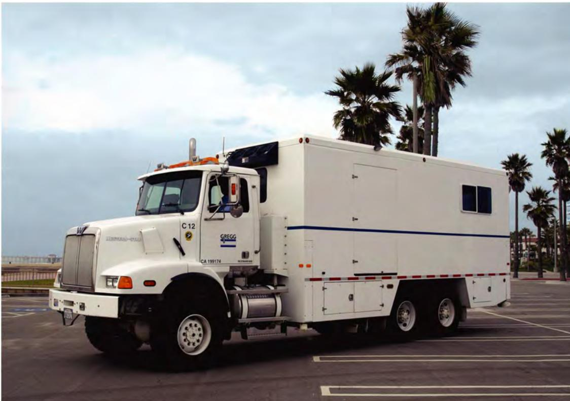
**Figure 10.** Truck mounted 250kN (25 ton) CPT unit
