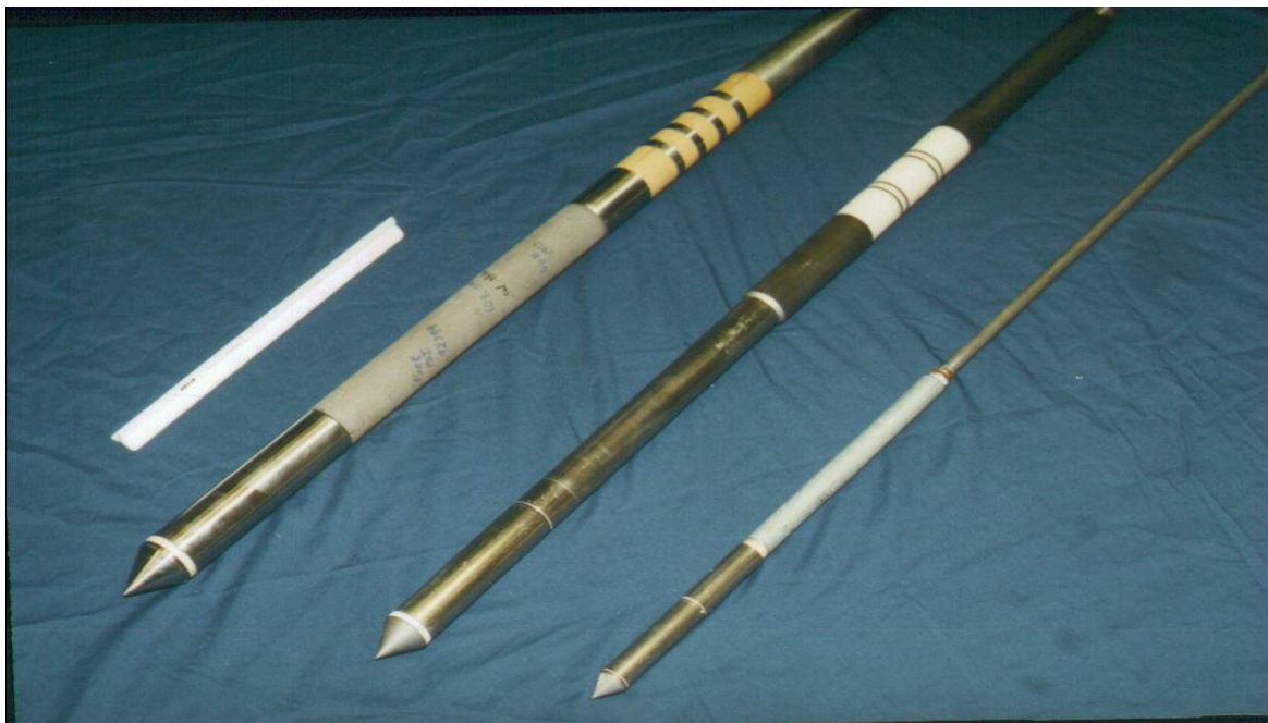
Figure 23 Example of some resistivity cones (courtesy P.Mayne)
