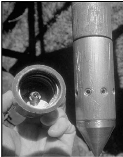
Figure 35 Waterloo profiler probe showing several sampling ports
