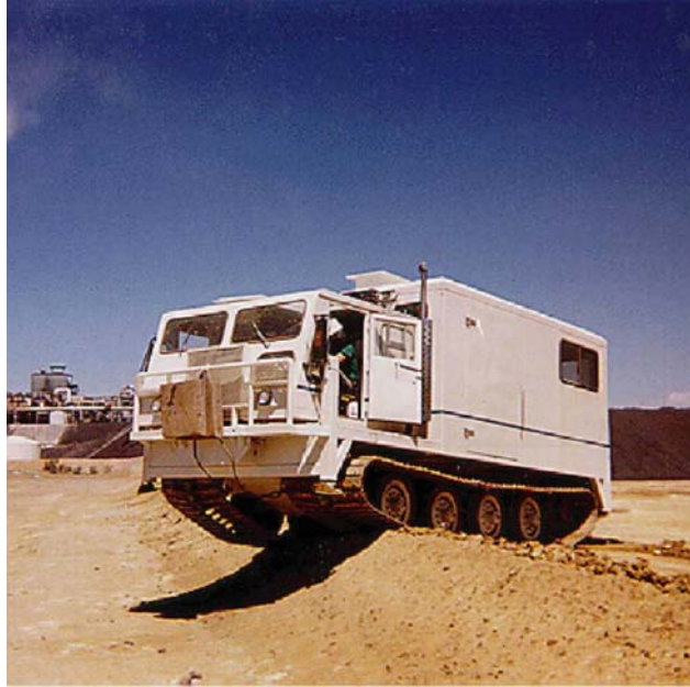
Figure 10 Track mounted 20 ton CPT unit
