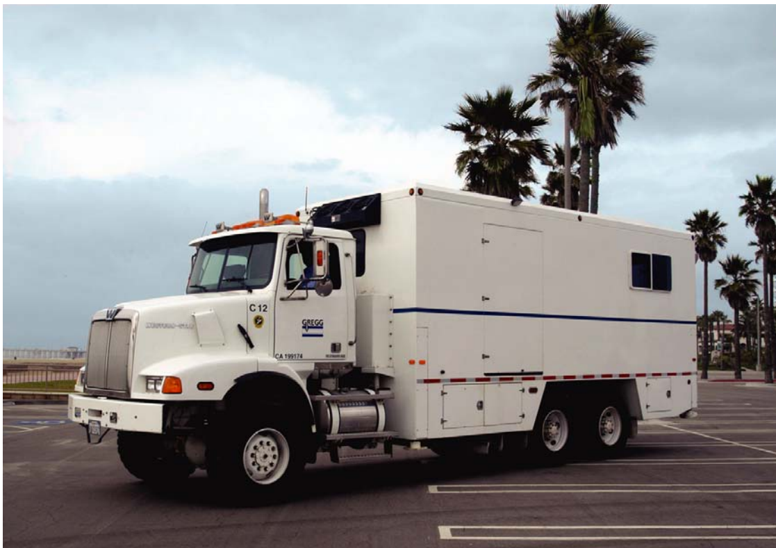
Figure 9 Truck mounted 25 ton CPT unit
