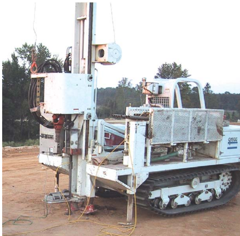
Figure 11 Small anchored drill-rig unit
