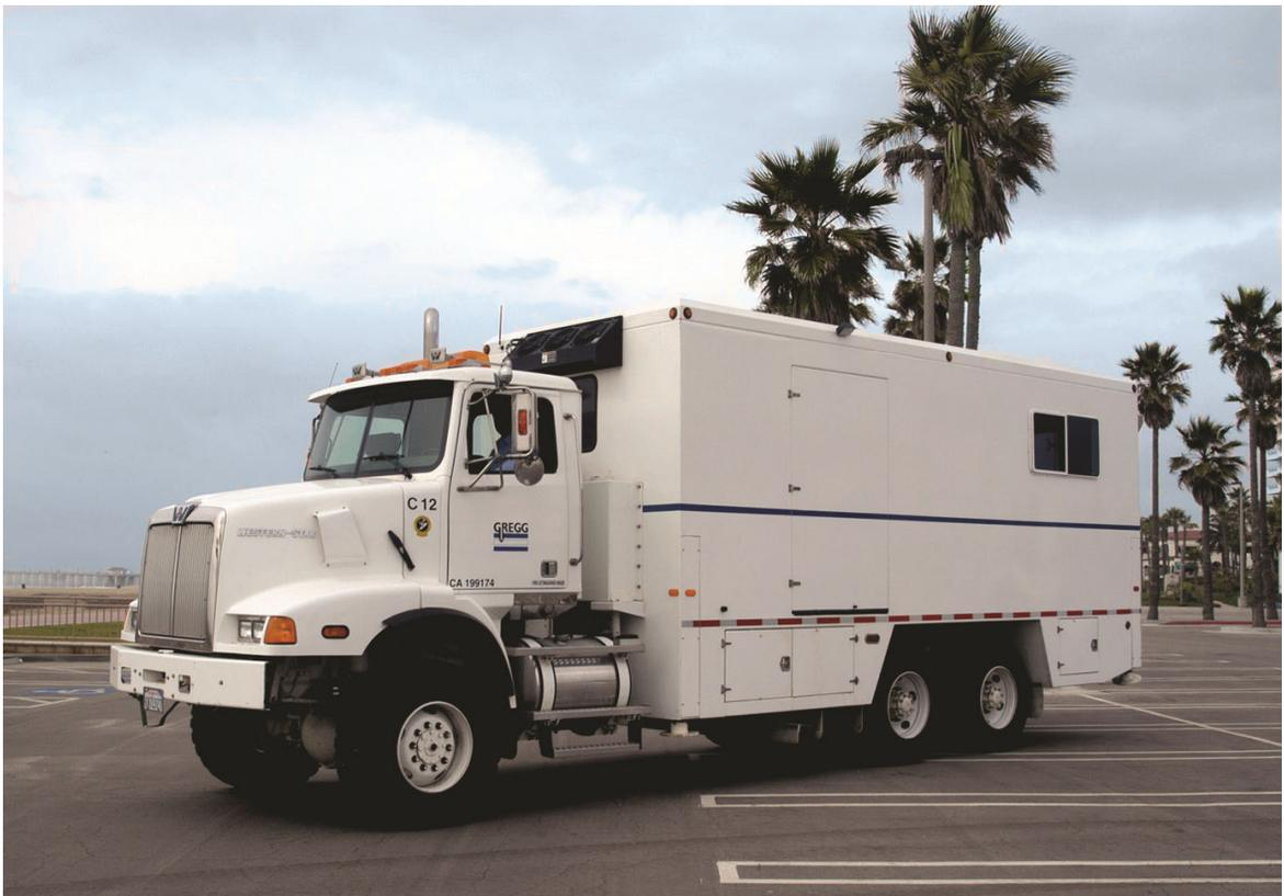
**Figure 9** Truck mounted 250kN (25 ton) CPT unit
