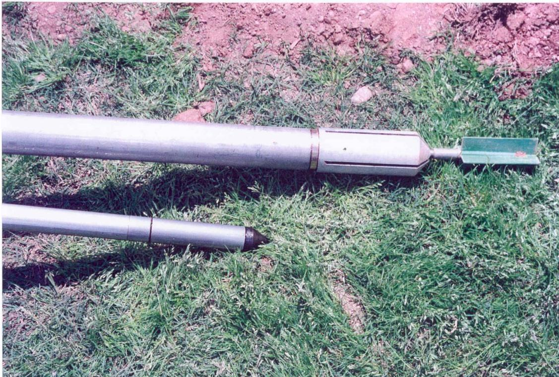
**Figure 33.** Typical field vane showing protective sheath for pushing in soft clays. A standard 10 cm<sup>2</sup> cone penetrometer is shown for scale.
