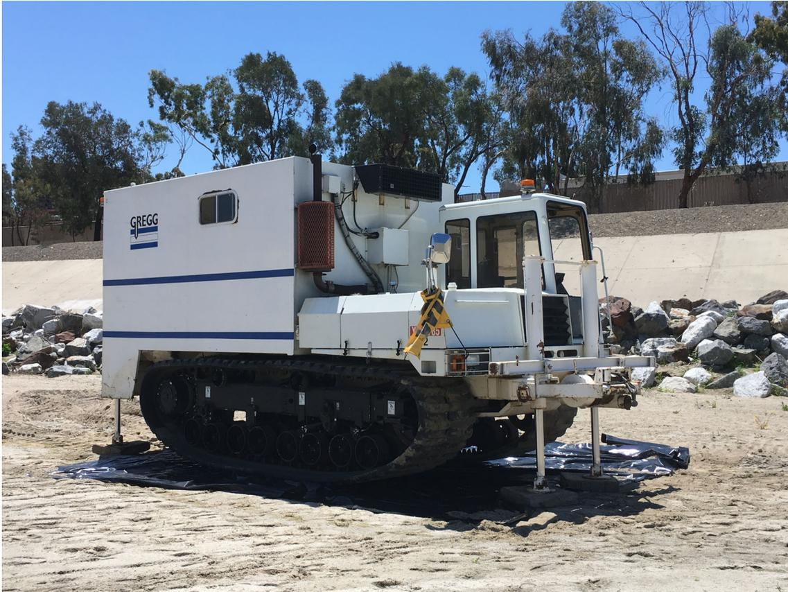
**Figure 10** Track mounted 200kN (20 ton) CPT unit
