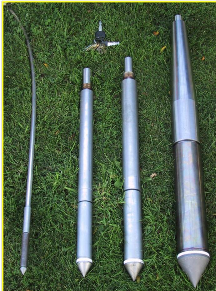
**Figure 7** Range of CPT probes (from left: 2 cm<sup>2</sup>, 10 cm<sup>2</sup>, 15 cm<sup>2</sup>, 40 cm<sup>2</sup>)
