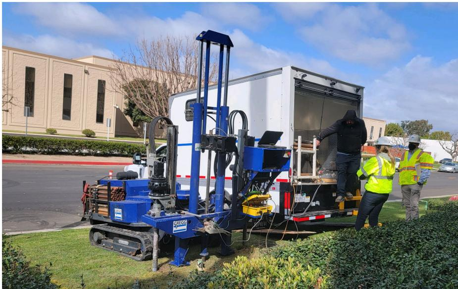
**Figure 11** Small anchored drill-rig unit
